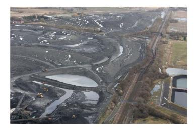
On Saturday, February 9, 2013, a train driver reported a "rough ride" along the Up Slow line between Doncaster to Scunthorpe, adjacent to Hatfield Colliery. Train services were carefully managed to protect public safety and the condition of the track deteriorated as evidence of large scale ground movement was observed.
